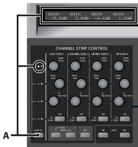
A. [DISPLAY] button (Selects which row displays parameters on the LCD display)
